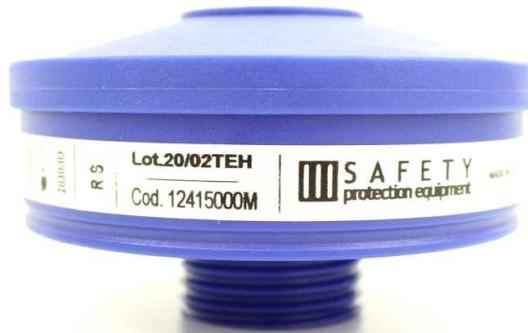
The 100 P3 R filter, with the standard thread connector (EN148-1, RD 40-1/7") can be used with the full face gas masks type SGE150, SGE 400/3 and SGE 400/3 BB, or equivalent and with the APA (Aria Protection adaptor) assembled on Ocean Reef snorkelling masks (Aria and UNO series). This filter protects against aerosols, particles, mist, fumes and dust.
